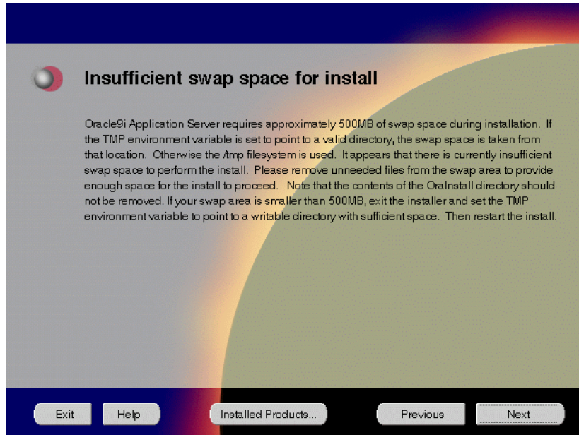
Figure 6–6 Insufficient Space in TMP Screen
