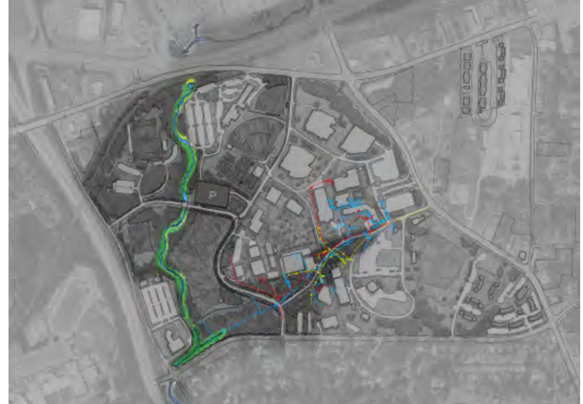
FIGURE 53: EXISTING UTILITIES IN THE LIBRARY LANE CORRIDOR. CURRENTLY, STORMWATER IS CONVEYED IN A PIPE ALONG LIBRARY LANE TO LINDSAY CREEK.
