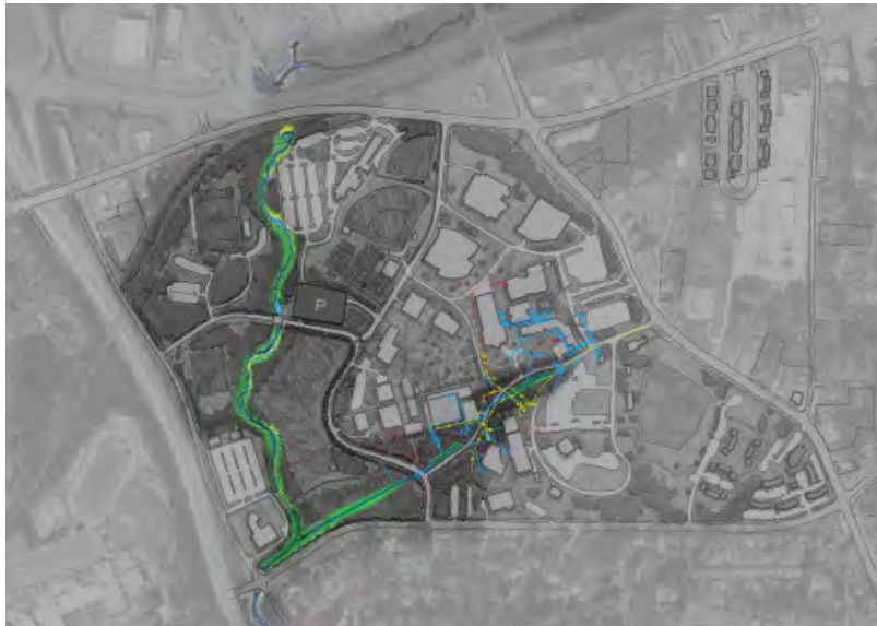
FIGURE 54: THE CREATION OF A SWALE IN THE LIBRARY LANE CORRIDOR WOULD ALLOW WATER QUALITY FILTRATION VIA SURFACE DRAINAGE EN ROUTE TO LINDSAY CREEK.
